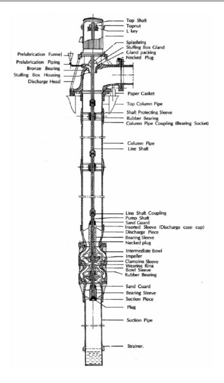
Figure – 2: Turbine Pump
