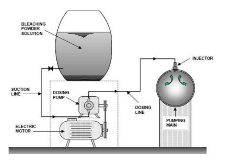
Figure - 5: Bleaching Powder Dosing Arrangement
